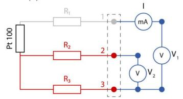
In this example, measure the voltage between terminals I and 3 (V<sub>1</sub>) and terminals 2 and 3 (V<sub>2</sub>), then measure the input current (I):
