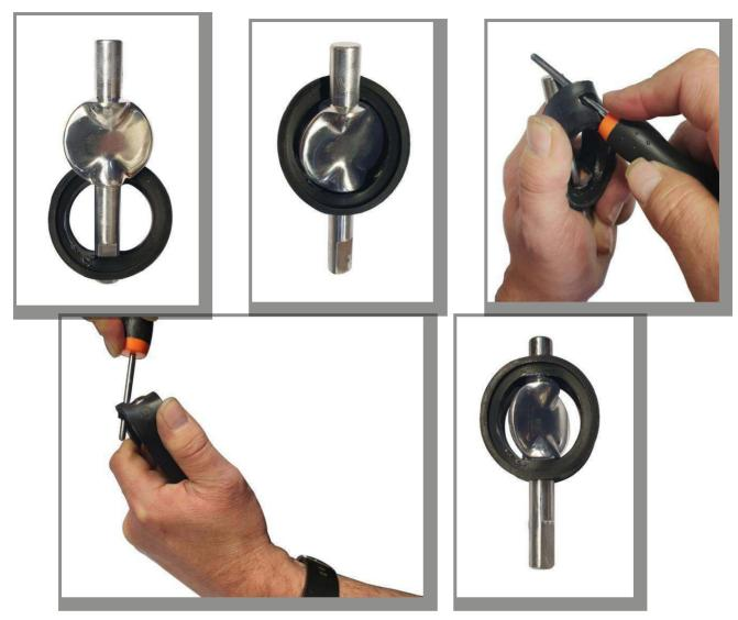
For valve's from DN65 and above, bend the seal manually without using any tools.
