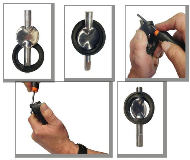
For valve's from DN63 and above, bend the seal manually without using any tools.
